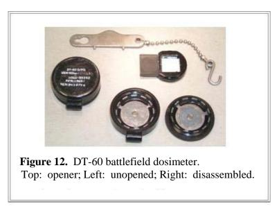
a. Passive dosimeter that uses a silver phosphate glass that darkens with exposure to high-energy gamma and thermal neutron irradiation. The dosimeter is housed in a black plastic case sealed with a rubber gasket.
